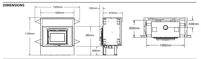
**ZERO CLEARANCE FRAMING** Cavity Height: 1600 mm Cavity Width: 1480 mm Cavity Depth: 610 mm
